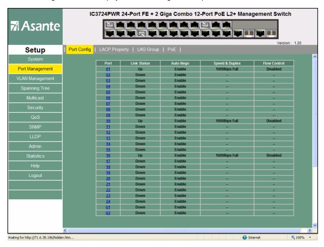
**Port Management – Port Config - Specific Port.** Settings can be made on a per port basis. When a port number is clicked the subscreen appears.
